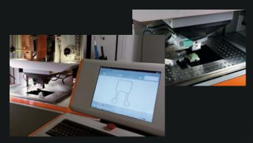
Designed for high autonomy, the CUT 1000 supports automated sequences with features including: dual 8 kg wire spools, long-lasting filters and deionizing systems, durable power feeds and wire guides, power failure restart capability, reliable workpiece results, an efficient wire chopper, and scheduled maintenance intervals.
